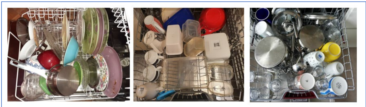
Fig. 7: Examples of dishwasher capacity use and limitations caused by dishware shape and variety (© Klingshirn et al.)
